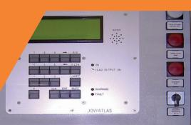
The supply rectifier TTC Wärtsilä JOVYREC HC16PS (PS = power supply) comes into use for external DC supply of conventional diesel-driven submarines. With the microprocessor-controlled rectifier of the type TTC Wärtsilä JOVYREC HC16PS it is possible to supply conventional submarines with DC voltage (shore connection rectifier). The supply rectifiers are manufactured customer-specifically according to the differentiated specifications of the respective type of submarine.
